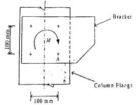
The shear force induced in the rivet A is
