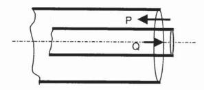
Densities of P and Q are 1000 and 800 kg/m $^3$  respectively. The average velocities of the liquids P and Q are 1 and 2.5 m/s respectively. The inner diameters of the pipes are 0.31 and 0.1 m. Both pipes are 5 mm thick. The ratio of the Reynolds numbers Re<sub>P</sub> to Re<sub>O</sub> is
