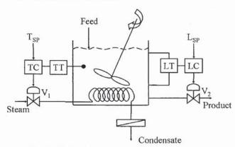
TC: Temperature controller, LC: Level controller, TT: Temperature transmitter, LT: Level transmitter, V1 and V2: Control valves
