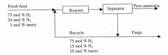
The single pass conversion for H<sub>2</sub> in the reactor is 20 %. The amount of H<sub>2</sub> lost in the purge as a **PERCENTAGE** of H<sub>2</sub> in fresh feed is
