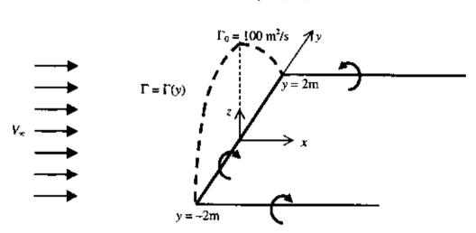
If the free stream velocity is 100 m/s, the induced angle of attack is
