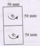
The torque balance equation (Bredt-Batho formula) for this section leads to
