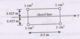
The wing root bending moment in steady level flight is  $M_y = 10$  N-m. If the airplane flies at a load factor n = 3.5, the maximum bending stress at the root is
