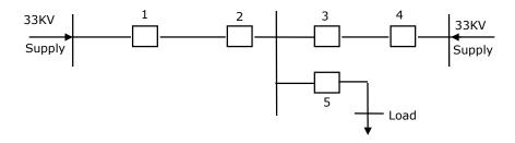
For proper fault discrimination directional over current relays will be required at locations
