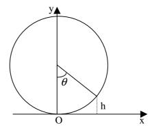
The 'London Eye' can be considered to be a circular frame of radius 67.5m on the circumference of which are 'capsules' carrying a number of people round the circle. Take a co-ordinate system where O is the base of the circle and Oy is a diameter. At any time after starting off round the frame, the capsule will be at height *h* metres when it has rotated  $\theta$ .<sup>o</sup>
