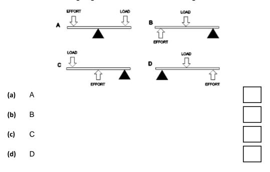
19 Which of the following diagrams shows a class 3 lever arrangement?
