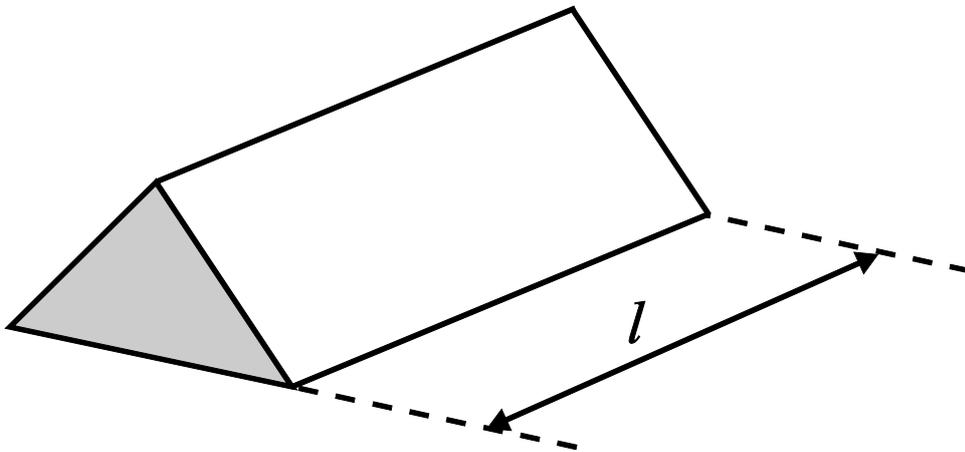
$$\text{Volume} = \text{area of shaded cross-section} \times l$$
