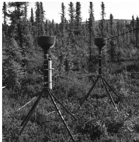
Passive air sampler containing a collector
