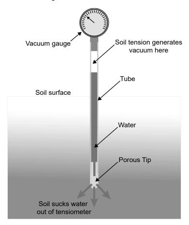
The tip of the tensiometer is made of porous ceramic.
