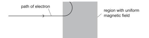
In the magnetic field, the electron follows a semi-circular path of diameter 0.0700 m.
