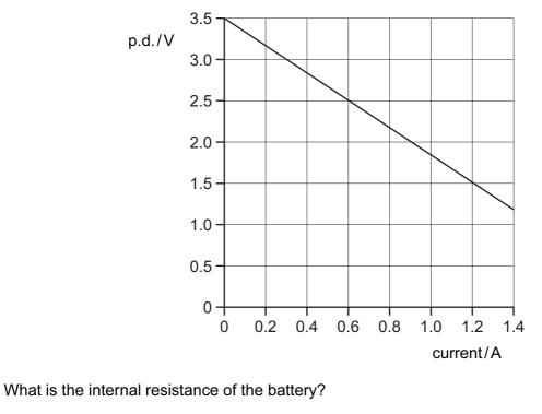
**A**  $0.60\Omega$  **B**  $1.2\Omega$  **C**  $1.7\Omega$  **D**  $2.3\Omega$
