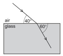
The angle between the ray and the edge of the glass block is 40° in the air and 60° in the glass. What is the speed of light in the glass block?
