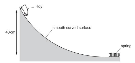
The toy, of mass 0.22 kg, runs down the curved surface through a vertical distance of 0.40 m. It strikes a spring of force constant  $350 \text{ Nm}^{-1}$  and compresses it a distance *x* before coming to rest.
