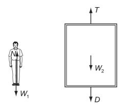
*N* is the force from the lift floor on the man.  $W_1$  is the weight of the man. *T* is the tension in the lift cable.  $W_2$  is the weight of the lift. *D* is the force from the man on the lift floor.
