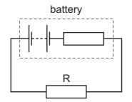
When 100 C flows around the circuit, 120 J of electrical energy is dissipated in resistor R and 20 J in the battery's internal resistance.
