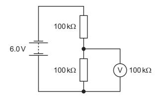
A voltmeter of resistance  $100 \text{ k}\Omega$  is connected across one of the resistors.
