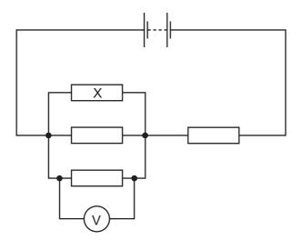
The voltmeter reads 6.0 V.The battery has negligible internal resistance.
