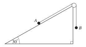
Particles A and B, each of mass  $m \log A$  are connected by a light inextensible string. Particle A rests on an inclined plane, particle B hangs freely, and the string passes over a smooth pulley at the top of the plane (see diagram).
