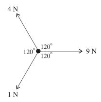
Coplanar forces of magnitudes 1 N, 4 N, 9 N act on a particle, as shown in the diagram; the angle between the directions of each pair of the forces is  $120^{\circ}$ . The resultant of the three forces has components X N parallel to the 9 N force and Y N perpendicular to the 9 N force.
