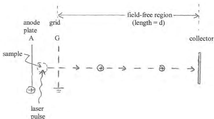
Fig. 9.1 A linear TOF mass spectrometer
