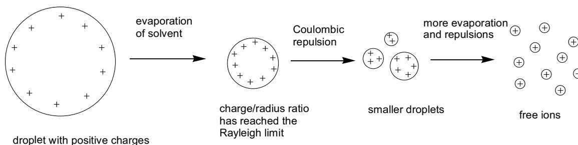
Fig. 9.2 The break-up of an electro spray
