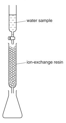
A  $50.0\,\mathrm{cm}^3$  sample of water containing dissolved calcium sulfate was passed through the ion-exchange resin. Each calcium ion in the sample was exchanged for two hydrogen ions. The resulting acidic solution collected in the flask required  $25.0\,\mathrm{cm}^3$  of  $1.00\times10^{-2}\,\mathrm{mol\,dm}^{-3}$  potassium hydroxide for complete neutralisation.
