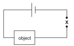
(a) Name a component which the boy can connect at **X** to show whether a current passes through the circuit.
