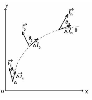
$\Delta l_n$  respectively. As the line segments are very small, the force over each segment can be considered constant.
