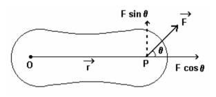
ineffective in producing rotational motion. The component,  $\overrightarrow{F}$  sin  $\theta$ , produces the rotational motion about the axis through O.
