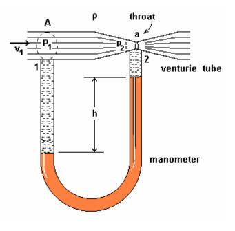
Using Bernoulli's theorem at points '1' and '2' which are at the same elevation,
