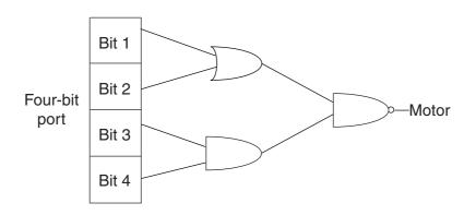
(i) The motor is switched ON when the final output from the circuit is 1.
