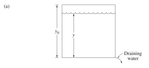
The diagram represents a vertical cylindrical water cooler of constant cross-sectional area A. Water drains through a hole at the bottom of the cooler. From physical principles, it is known that the volume V of water decreases at a rate given by
