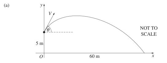
An angler casts a fishing line so that the sinker is projected with a speed  $V \text{ m s}^{-1}$  from a point 5 metres above a flat sea. The angle of projection to the horizontal is  $\theta$ , as shown.
