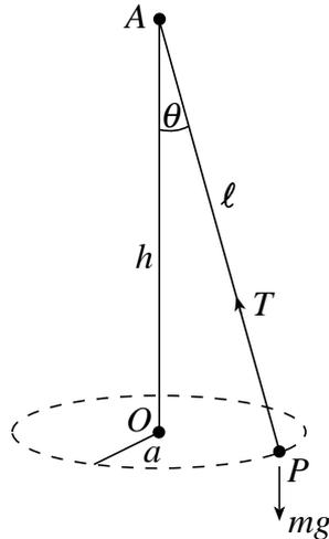
A conical pendulum consists of a bob  $P$  of mass  $m$  kg and a string of length  $\ell$  metres. The bob rotates in a horizontal circle of radius  $a$  and centre  $O$  at a constant angular velocity of  $\omega$  radians per second. The angle  $OAP$  is  $\theta$  and  $OA = h$  metres. The bob is subject to a gravitational force of  $mg$  newtons and a tension in the string of  $T$  newtons.
