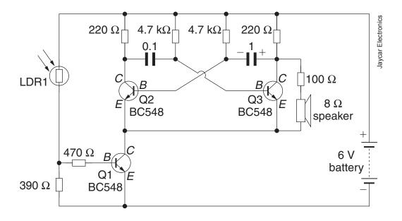
Propose and explain a fault-finding sequence for testing this circuit if the speaker does not produce an output.
