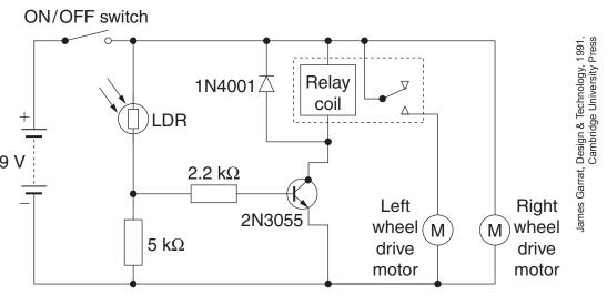
Outline how this vehicle will behave when the ON/OFF switch is turned on.
