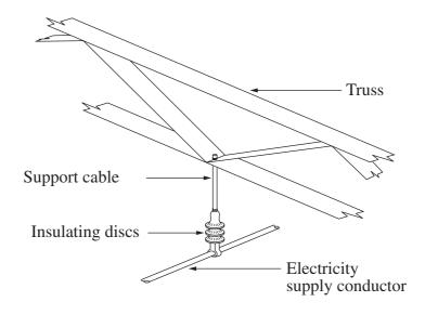
(i) The support cable must not extend more than 0.5 mm when placed under the maximum tensile force. Calculate the maximum allowable length of the support cable.
