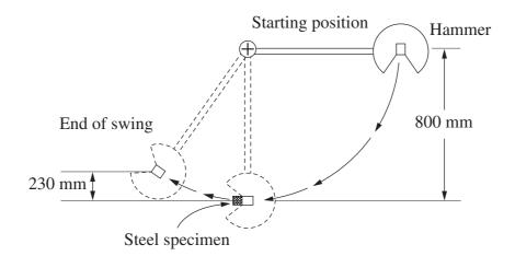
Assuming that there is no friction loss in the test machine, determine the energy lost by the hammer in fracturing the steel specimen.
