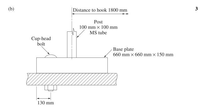
Determine the force in EACH of the TWO bolts if a 90 kg sailor is lifted with the hoist.
