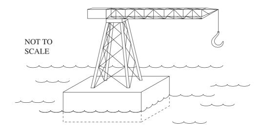
Determine the load on the crane that would submerge 70% of the pontoon below the surface of the water. (Assume that the pontoon remains level.)
