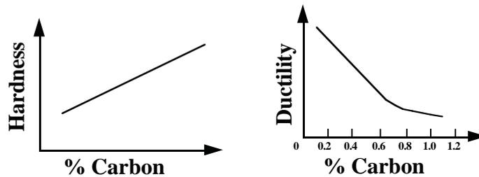
Most candidates answered this section quite well, showing hardness increasing with carbon content and ductility decreasing as carbon increases.
