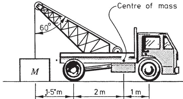
**(i) Determine the maximum load, M, that could be safely lifted by this tow truck.**
