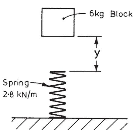
$$\Delta PE = \Delta \text{Strain Energy/Spring}$$
