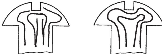
Indicates flow lines proceed fully around head of bolt. Example indicates the slot to be stamped.
