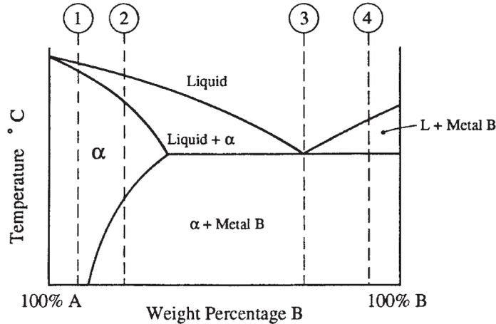
(i) Alloy 2 and alloy 3 are cooled under equilibrium conditions to room temperature. Draw and label the resulting microstructures.
