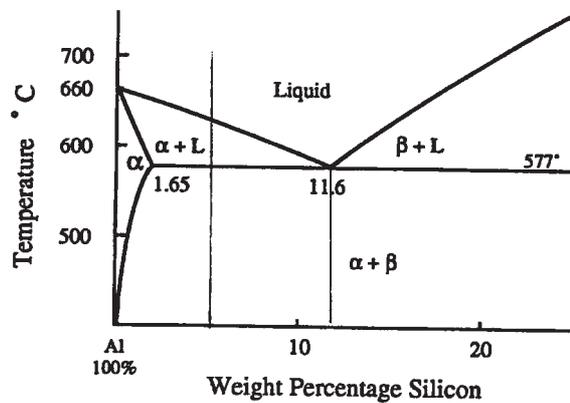
(i) Two alloys, a 95% aluminium–5% silicon alloy, and an 88.4% aluminium–11.6% silicon alloy, are cooled under equilibrium conditions to room temperature. Draw and label the resultant microstructure for each of the alloys.
