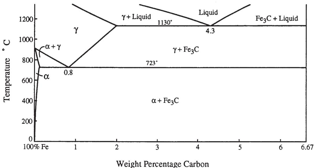
A sample containing 0.4% carbon is cooled under equilibrium conditions from 900°C to room temperature. Draw and label the microstructure at 750°C, and the microstructure at room temperature.
