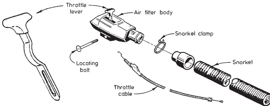
(a) The air filter body is made from high-density polyethylene.
