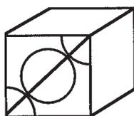
$$\begin{aligned} d &= 4 \times r \\ &= 4 \times 1.431 \\ &= 5.724 \text{ \AA} \end{aligned}$$
