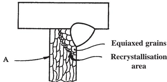
*Heat affected zone clearly shown as being different to the parent metal.*
