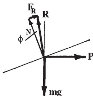
$$\begin{aligned} P &= mg \tan 11.47^\circ \\ &= 120 \times 9.8 \tan 11.47^\circ \\ &= 238.6 \text{ N} \end{aligned}$$
