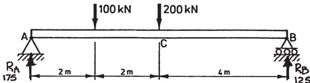
(i) Calculate the reactions at A and at B.
