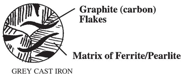
Drawings were generally well done, but the labels were often omitted or incorrect. The matrix in a grey cast iron can vary with composition, inoculants, and cooling history. The matrix can vary from a fully pearlitic structure to areas of ferrite and pearlite.
