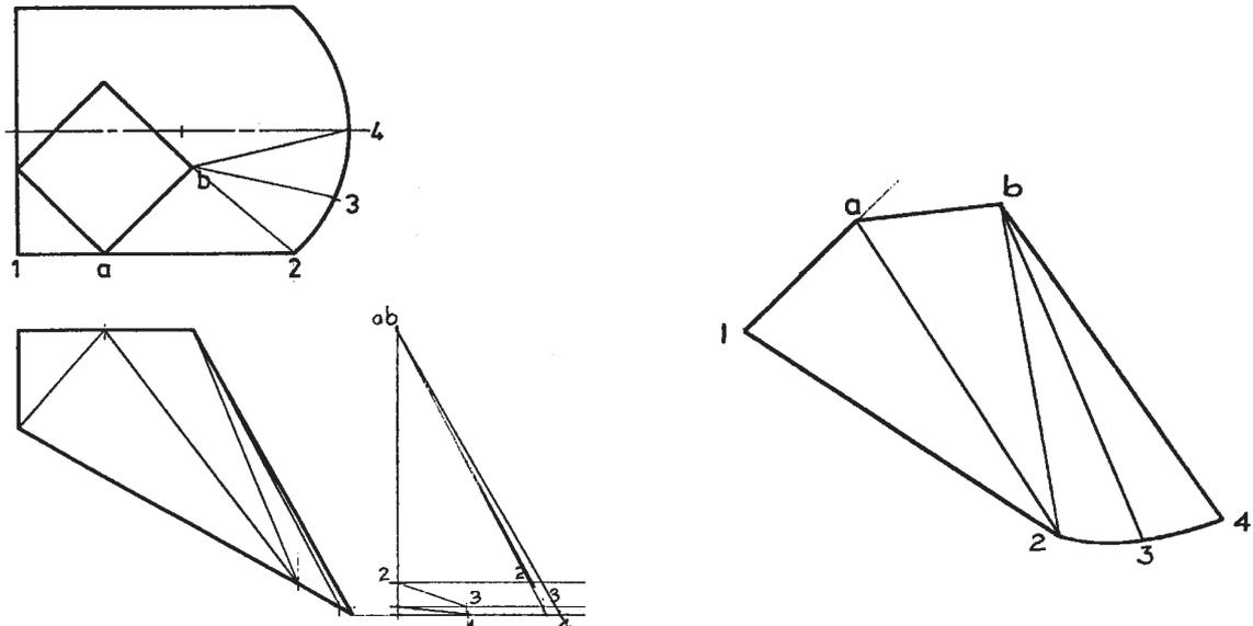
The question was generally well attempted with many candidates scoring maximum marks. Most problems occurred with the varying heights in the true length diagram and failure to determine the true lengths of lines 2,3 and 3,4. Curved edges in the drawing should be drawn as a curve on the development.
