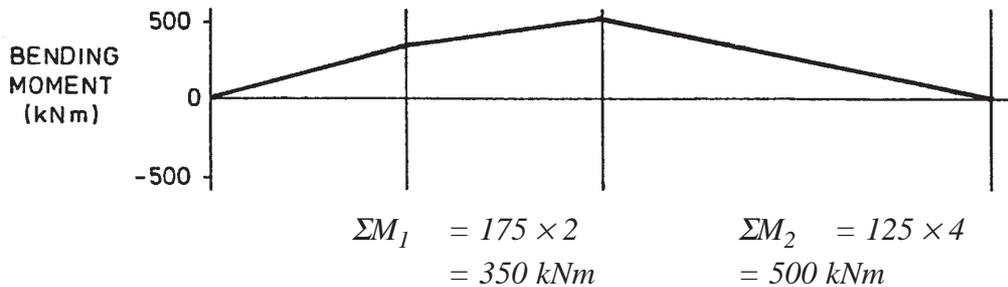
Most candidates recognised that a simply supported beam has zero bending moments at each end, and were able to take a moment equation at the points of loading to find the value of the moment. Most plotted the BM as a straight line, as only point loads were being applied. Many did not show the correct sign of BM (+ve) even though this is critical to BM calculations.
