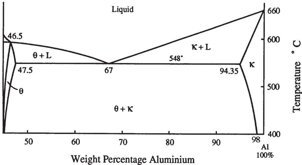
The maximum solubility of copper in aluminium is 5.65% and occurs at 548°C. The eutectic composition is 67% Al–33% Cu and the eutectic temperature is 548°C.
