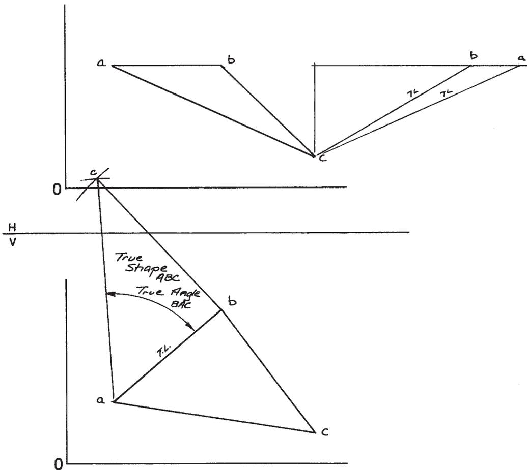
An alternative solution, which included a part mathematical solution, shows working and the correct solution. This method is not preferred but was acceptable for full marks. Another common error was made when candidates measured the apparent angle BAC and gave this as the solution, or failed to use any suitable method of construction to find true shape of the triangle to in turn find true angle. Others produced the true shape of the triangle but failed to measure the angle as 52°.
