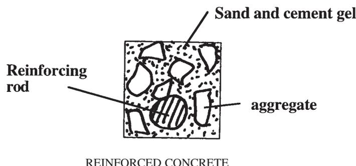
The key elements of reinforced concrete that markers were looking for was reinforcing steel, coarse aggregate and fine aggregate held together by a cement gel. Some sketches and labels were very poor, indicating only 'reinforcing' and 'concrete', the information given in the question.
