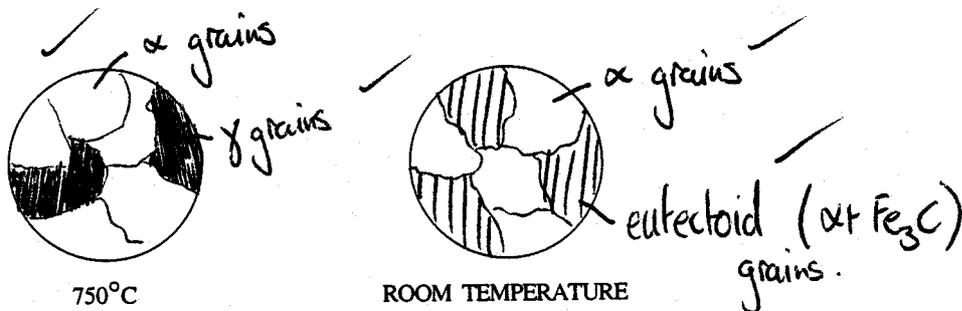
Room temperature microstructure was generally well drawn, but labels reflected some confusion with eutectic and eutectoid, and  $\text{Fe}_3\text{C}$  phase rather than ' $\alpha$  and  $\text{Fe}_3\text{C}$ '.
