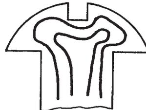
Indicates flow lines proceed fully around head of bolt. Example indicates the slot to be stamped.
