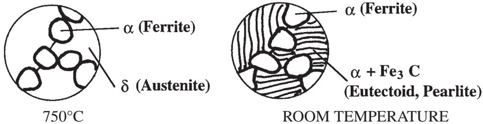
Microstructures at 750°C caused difficulty to some candidates, who included liquid phase and/or dendrites. Many had difficulty drawing austenite as an equiaxial grain structure. Eutectoid type structures were common. The phase field involved is  $\alpha$  and  $\gamma$  (ferrite and austenite), and these are the only two phases that can be present for the stated circumstances. The ferrite precipitates from the austenite along the grain boundaries of the austenite.
