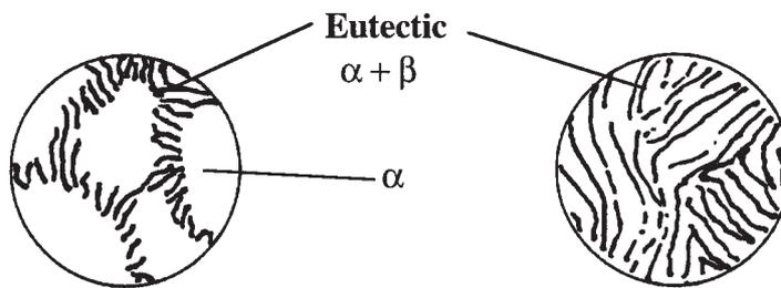
95% ALUMINIUM–5% SILICON    88.4% ALUMINIUM–11.6% SILICON
