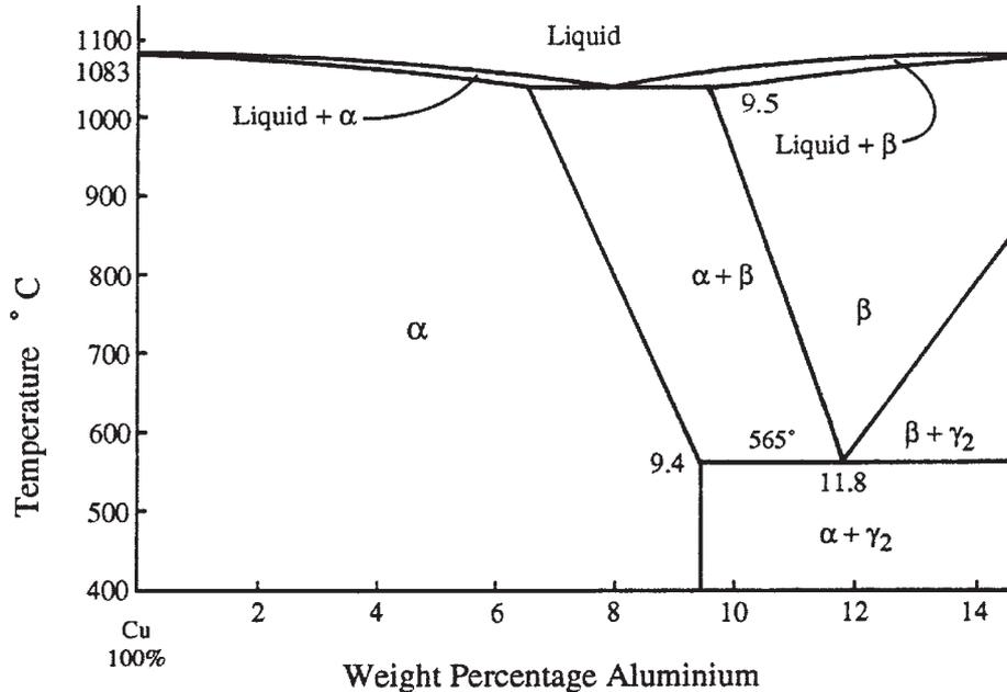
The maximum solubility of aluminium in copper is 9.4% and occurs at 565°C. The eutectoid composition is 88.2% Cu–11.8% Al and the eutectoid temperature is 565°C.
