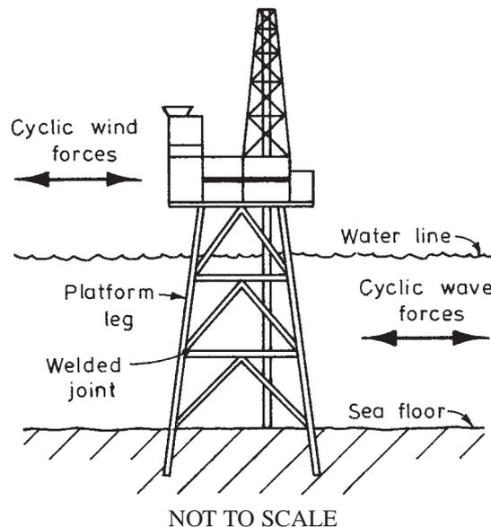
**(i) Name and describe the type of corrosion that would occur at the cracked welded joints.**
