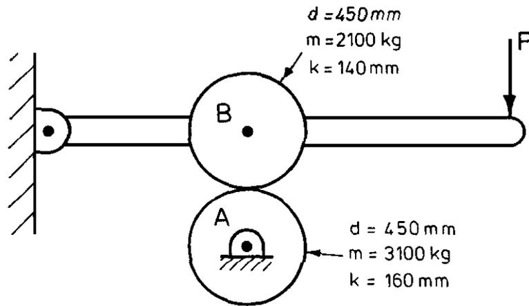
A force  $P$  is applied to bring the rollers together, so that a normal force of 20 kN is acting between the rollers.
