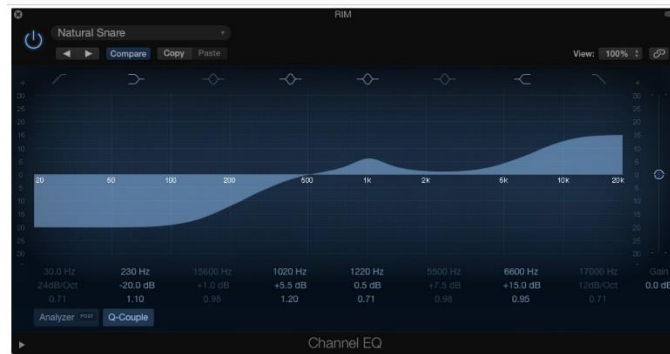
Image: Better practice of equalisation to enhance snare drum, remove rumble, improve clarity and brightness (backed up by written explanation)
