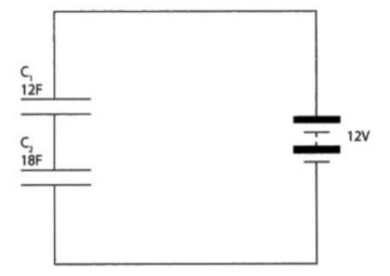
Calculate the total capacitance of the two capacitors.
