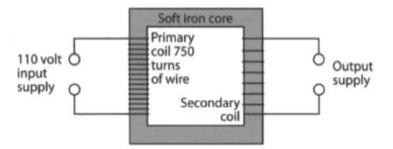
A peak voltage of 34 V is required as the output from the transformer.
