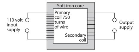
A peak voltage of 34 V is required as the output from the transformer.
