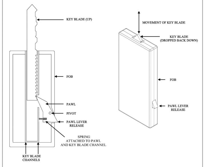
Fob dimensions: Depth = 10 mm, Width = 40 mm, Height = 85 mm
