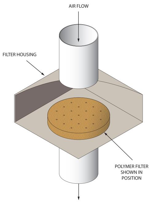
FILTER HOUSING DIMENSIONS L175mm W175mm H65mm FILTER HOUSING WITH PIPEWORK
