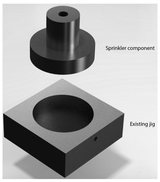
Jig dimensions: L= 56 mm, W= 56 mm, H=20 mm
