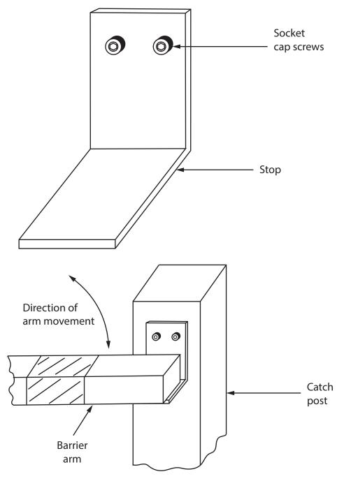
Stop Dimensions: L = 110 mm, W = 60 mm, H = 105 mm
