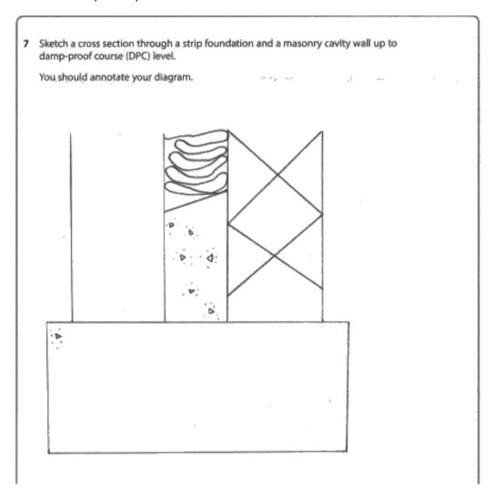
Although the candidate has not labelled the components of the concrete foundation, three components have been correctly detailed. The concrete foundation, cavity wall fill and internal blockwork are all awarded one mark each. No marks are awarded for the external brickwork as it has no fill pattern and has not been annotated.
