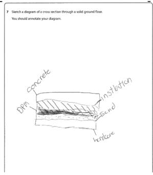
5 marks were awarded for this response. Although the sketch is of a poor quality, 5 components of a solid ground floor are indicated and the correct order.
