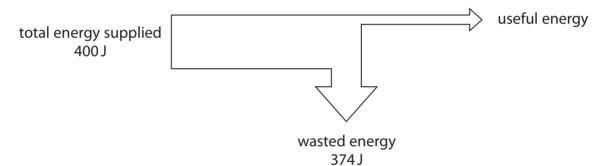
Calculate the efficiency of the machine.
