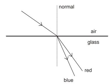
Red light travels at speed *c* in air, but only 2c/3 in glass. Red light has a wavelength of  $\lambda$  in air.
