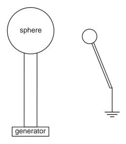
The surface area of the large sphere is  $0.04m^2$ , and it discharges by sparking to the small sphere when the charge density on the large sphere reaches  $0.25 \text{ C/m}^2$ .
