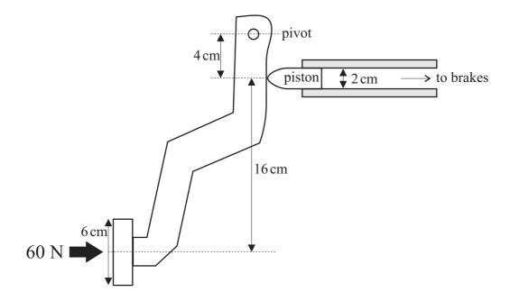
A driver applies a force of 60 N to the pedal. What force is applied to the piston?
