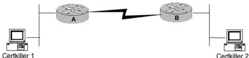
Certkiller 1 and Certkiller 2 are on Ethernet LANs in different buildings. A serial line is installed between two Cisco routers using HDLC serial line encapsulation. Routers A and B are configured to route IP traffic. Certkiller 1 sends a packet to Certkiller 2. What is the destination MAC address of the packet on Certkiller 1's Ethernet?
