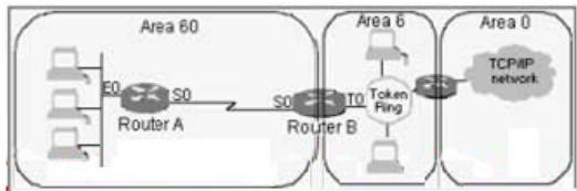
In a reorganization, OSPF areas are realigned. Is this a valid network design? If not, which changes could be made to the network and/or router configuration? (Choose two)
