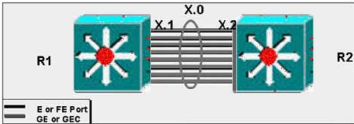
L3 switches R1 and R2 are in the backbone of the network. They are connected by a routed EtherChannel bundle consisting of eight Gigabit Ethernet ports. The routed link is represented as subnet X.0 in the diagram. Since X.0 is routed, it is not a VLAN trunk. How can spanning tree loops be prevented in the backbone of this network?
