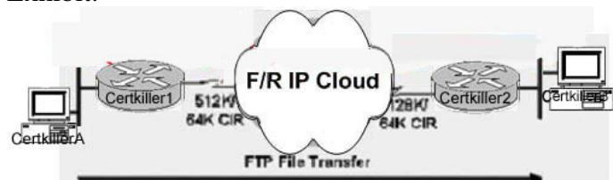
Router Certkiller 1 has a 512K-access port into the frame relay cloud. Router Certkiller 2 has 128K-access port into the frame relay cloud. The two routers are connected with symmetrical PVCs that are configured for 64K committed information rate (CIR). What Frame Relay Traffic Shaping map-class
