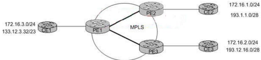
In the MPLS network shown, which subnets would be in the same Forwarding Equivalence Class (FEC) on router PE1:
