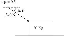
28. The normal force acting on the block is \_\_\_\_N.
