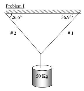
The two cables are used to suspend a 50 Kg object below the ceiling. Find the tension in each cable.
