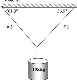
The two cables are used to suspend a 105 Kg object below the ceiling. Find the tension in each cable.
