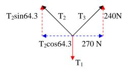
Items #14 and #15 can be answered directly from the diagram. The tension in cable #2 can be found from the horizontal forces equation.
