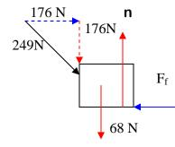
From  $\Sigma$  F<sub>Y</sub>: **n** – 68N – 176 N = 0 **n** = 244 N From  $\Sigma$  F<sub>X</sub>: 176N – F<sub>f</sub> = 0 F<sub>f</sub> = 176 N
