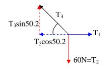
From  $\Sigma$  F<sub>Y</sub>: T<sub>3</sub>sin50.2 - 60 = 0 T<sub>3</sub> = 60/sin(50.2) = 78.1 N From  $\Sigma$  F<sub>X</sub>: T<sub>1</sub> - T<sub>3</sub>cos(50.2) = 0 T<sub>1</sub> - {78.1}cos(50.2) = 0 T<sub>1</sub> = 50 N
