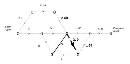
Another appropriate diagram for the stated conditions is shown below. This diagram shows that J must wait for both G and I to finish before starting. Importantly, it indicates that G is still also a predecessor of H and that D and F are not predecessors of J. However, not many students answered this way.
