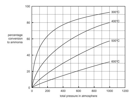
**a.** A particular industrial plant uses a pressure of 300 atm and a temperature of 500°C. From the graph, determine the percentage yield of ammonia under these conditions.
