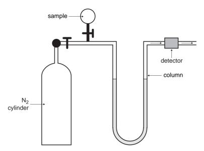
**a.** Clearly identify, on the diagram, the mobile and stationary phases in the gas chromatograph shown and explain how gas chromatography is able to separate the components of a gaseous mixture.
