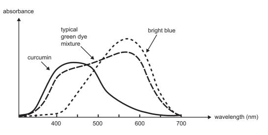
UV-visible spectroscopy is used to analyse the curcumin content of tinned peas.
