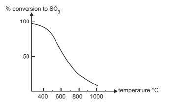
There is almost complete conversion of sulfur dioxide to sulfur trioxide at 300°C. However, this reaction is performed at a higher temperature of approximately 450°C in industry. Why?
