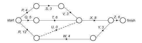
The activities and their completion times (in hours) that are needed to complete a project are shown in the network above.
