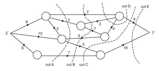
On the directed graph above, the values on the edges give the maximum flow between nodes in the direction of the arrows.
