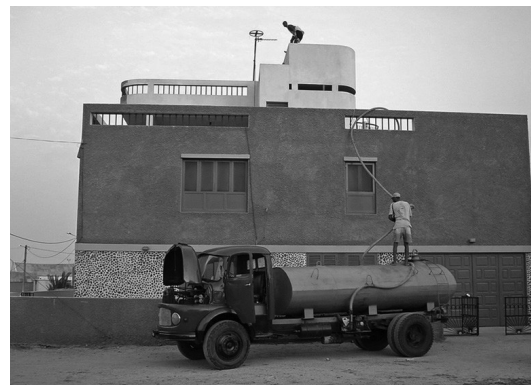
Drinking water being delivered to a home on the island of São Vicente. The water is stored in a water tank on the roof.
