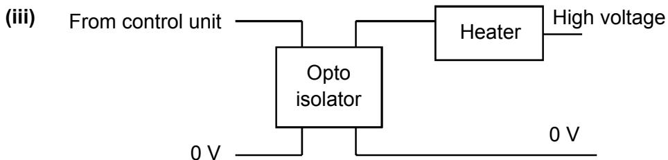
Electrical isolation is achieved because there is no physical connection between the two circuits. Therefore the transfer of the signal can occur without any interference from the high voltage circuit. [4]
