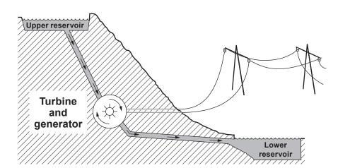
The hydroelectric power station is only used when we need more electricity than the rest of the power stations around the country can supply.
